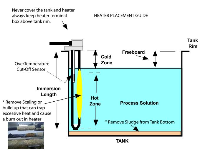
Always keep a minimum of at least 2" inches of solution level above Heater Hot Zone
